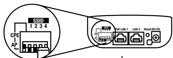
b) Make sure switches 1 to 4 are positioned identically on all the antennas.
